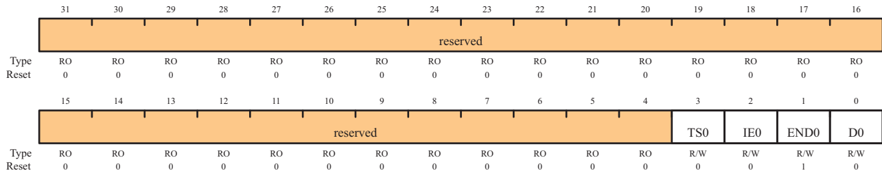
ADC Sample Sequence Control 3 (ADCSSCTL3)
