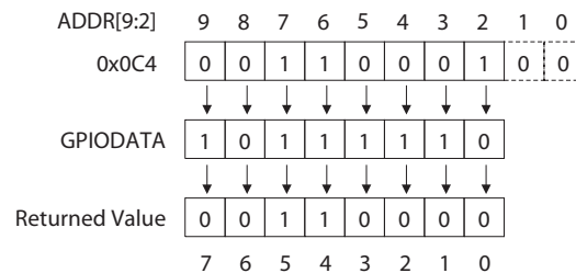
Figure 8-4. GPIODATA Read Example
