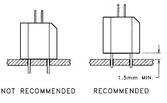
Good printed circuit board layout avoids putting any spreading (plastic under tension) force on the leads of the LED and photocell.
