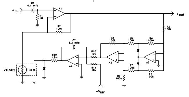
Figure 9. AGC Circuit with Electrical Setpoint
