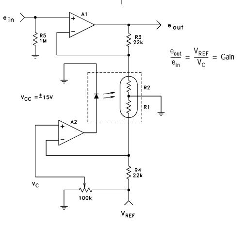
Figure 10. Electrically Programmable Gain
