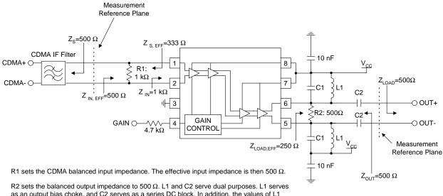
R2 sets the balanced output impedance to 500  $\Omega$ . L1 and C2 served dual purposes. L1 serves as an output bias choke, and C2 serves as a series DC block. In addition, the values of L1 and C2 may be chosen to form an impedance matching network of the load impedance is not 500  $\Omega$ . Otherwise, the values of L1 and C1 are chosen to form a parallel-resonant tank circuit at the IF when the load impedance is 500  $\Omega$ .
