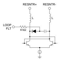
To tune the VCO the designer only needs to calculate the value of the inductors connected to pins 18 and 20 (RESNTR- and RESNTR+). The inductor value is determined by the following equation.
