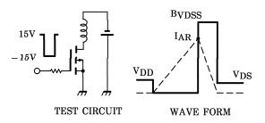
$$\begin{array}{ll} Peak~I_{AR} = -18A,~R_G = 25\Omega & E_{AS} = \frac{1}{2} \cdot L \cdot I^2 \cdot (\frac{B_{VDSS}}{B_{VDSS} - V_{DD}}) \end{array}$$
