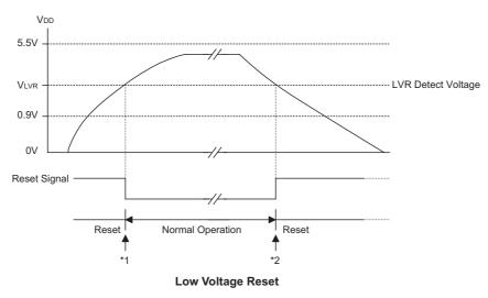
Note: \*1: To make sure that the system oscillator has stabilized, the SST provides an extra delay of 1024 system clock pulses before entering the normal operation.
