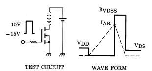
$R_G$  = 25  $\Omega$  $V_{DD}$  = 90 V, L = 48.4 mH  $EAS = \frac{1}{2} \cdot L \cdot I^{2} \cdot \left( \frac{BVDSS}{BVDSS - VDD} \right)$
