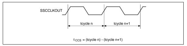
Figure 1 Cycle to cycle jitter (SSCCLKOUT)
