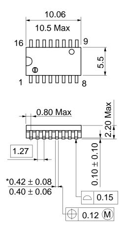
\*Dimension including the plating thickness Base material dimension
