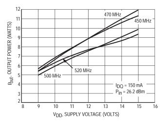
Figure 8. Output Power versus Supply Voltage
