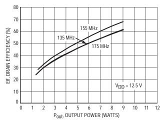
Figure 23. Drain Efficiency versus Output Power
