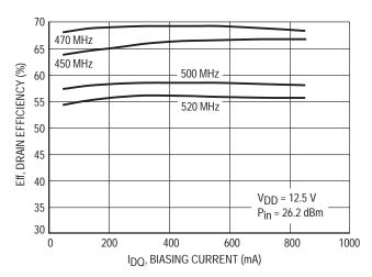
Figure 7. Drain Efficiency versus Biasing Current
