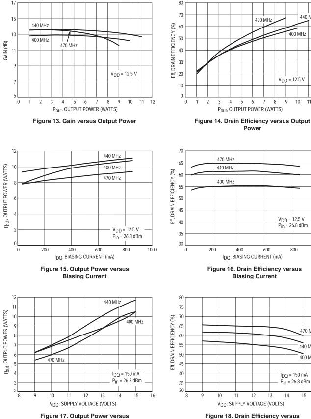
Figure 18. Drain Efficiency versus **Supply Voltage**
