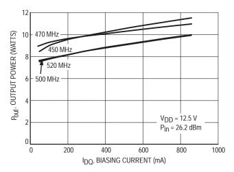
Figure 6. Output Power versus Biasing Current
