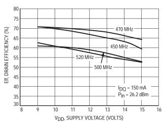
Figure 9. Drain Efficiency versus Supply Voltage
