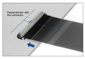
To assure correct electrical and mechanical connection do not insert FPC at angle. It must be fully inserted.
