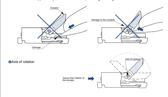
The actuator will rotate 135 degrees maximum. Do not apply force to rotate further.
