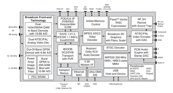
The **BCM7110** is a single-chip set-top box device that combines the key aspects required for the next generation of set-top boxes including cost-effective single-chip design, personal video recording (PVR), broadband communication via DOCSIS™ 1.1 cable modem, and support of all major global standards for worldwide deployment.
