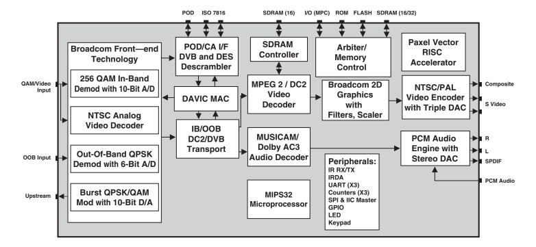
The **BCM7100** is a cable set-top box system on a single chip, integrating Broadcom's field-proven BCM3120 cable transceiver technology, BCM7010 MPEG/AC-3 decoder technology, BCM7014 advanced 2D/3D graphics and system integration technology, BCM3310 MIPS microprocessor technology, all key interfaces to external memory and I/O, and the necessary peripherals for set-top box applications.
