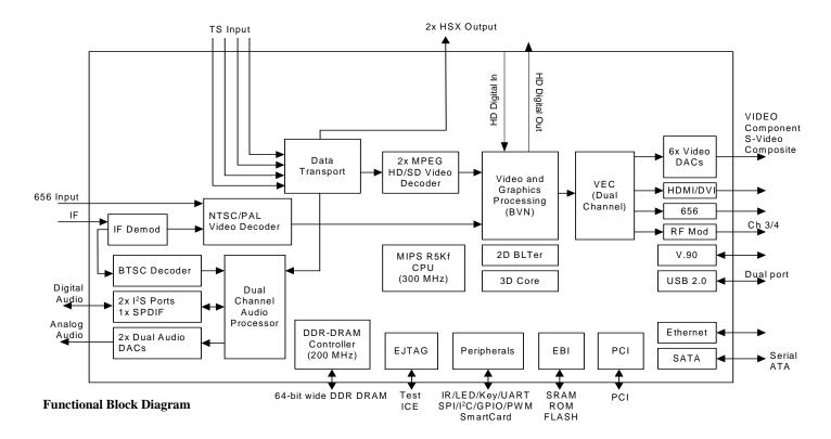
The **BCM7038** combines an IF demodulator, an NTSC/PAL video 3D Y/C comb filter enabled decoder, a transport processor, dual digital audio processors, dual high-definition (HD) MPEG video decoders, advanced 2D and 3D graphics processing, digital processing of analog video and audio, analog video digitizer and DAC functions (six DACs), stereo high-fidelity audio DACs, an MIPS R5000 class processor, and a peripheral control unit providing a variety of set-top box control functions.
