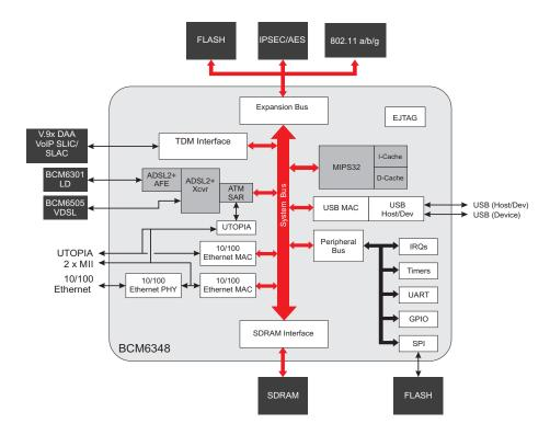
The BCM6348 combines a G.992.1/G.992.2/G.992.3/G.992.5/ T1.413 ADSL transceiver and AFE with a high-performance MIPS32 CPU, two 10/100-Mbps Ethernet interfaces, USB (host/device) transceiver, expansion bus interface supporting PCI, mini-PCI, CardBus, and PCMCIA into a single, high-performance chip.
