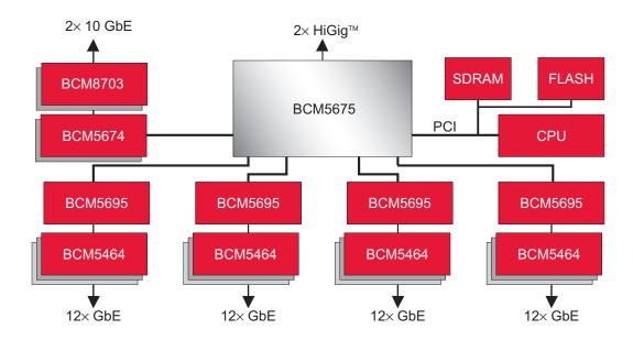
The BCM5674 10-Gigabit Ethernet switch is a scalable, multilayer switch-on-chip member of the StrataXGS family. The BCM5674 is a dual-port switch, which supports a 10 Gigabit Ethernet (IEEE 802.3ae) port and a HiGig<sup>TM</sup> uplink port. The 10 Gigabit Ethernet port can be used to interface to the XENPAK module via the XAUI interface.
