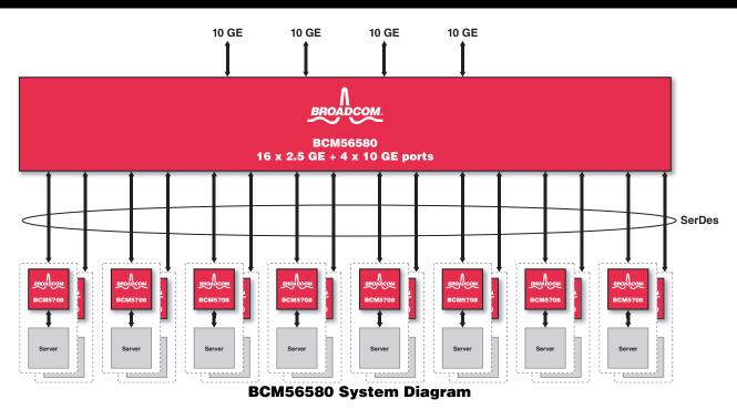
The BCM56580 network switch is a high-density, 2.5-Gigabit Ethernet switching chip solution with 20 ports. Additionally, the BCM56580 integrates all the SerDes required to interface to applicable copper and fiber physical interfaces. The integrated SerDes functionality includes 10-Gbps XAUI interfaces and 2.5/1-Gbps SGMII PHY interfaces. The integrated SerDes complies with the CX-4 standard and PICMG3.1 standard, which ensures interoperability with Ethernet line cards in an advanced TCA chassis.
