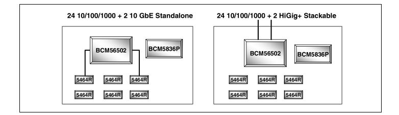
The BCM56502 is the fifth generation of the highly-integrated and costeffective StrataSwitch and StrataXGS product line and is a single-chip solution with 24-GbE ports and two 10-GbE/HiGig+ uplink ports.
