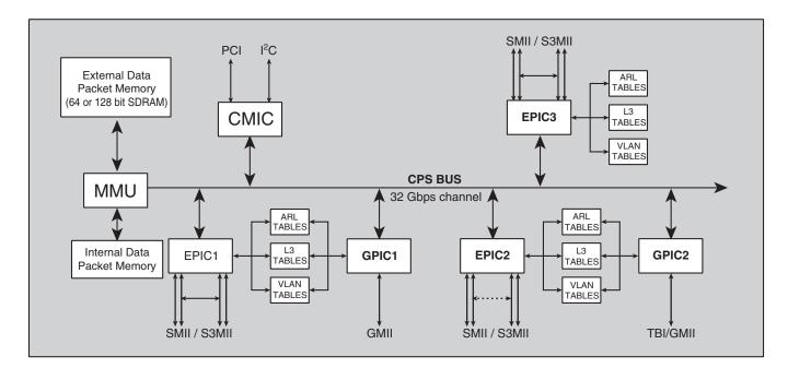
The **BCM5615**, with a forwarding rate of 6.6 Mpps, defines the next generation of performance for single-chip switching solutions. Through its advanced ContentAware<sup>TM</sup> feature set, the StrataSwitch II<sup>TM</sup> product family supports advanced applications and services, at wire speed, with nonblocking performance.
