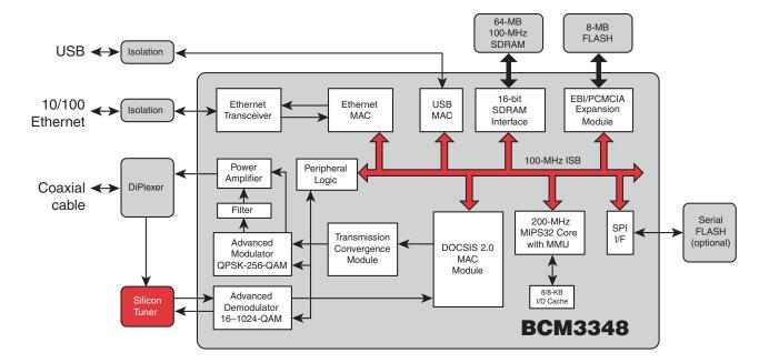
The BCM3348 combines an RF receiver with an advanced QAM and S-CDMA demodular, an advanced QAM transmitter, a complete DOCSIS 2.0 Media Access Controller (MAC), a 200-MHz MIPS32™ communication processor, a 16-bit, 100-MHz SDRAM interface, 10/100 Ethernet MAC with integrated transceiver and MII Interface, and a medium-speed USB 2.0 controller with integrated transceiver.
