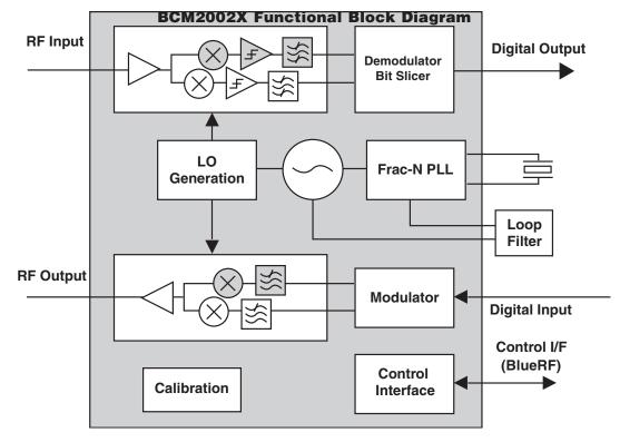
The **BCM2002X** is a Bluetooth 1.1 compliant integrated radio transceiver device operating in the 2.4 GHz band. It is ideal for integration in mobile phone applications where the radio has been designed to handle the harsh environments of mobile phones to provide the highest communication link quality of service.
