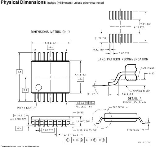
Dimensions are in millimeters
