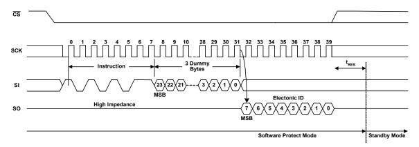
Figure 27. Release from Software Protection and Read Electronic Signature (RES) Instruction Sequence
