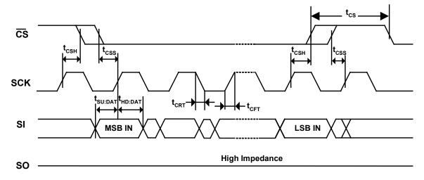
Figure 4. SPI Mode 0 (0,0) Input Timing
