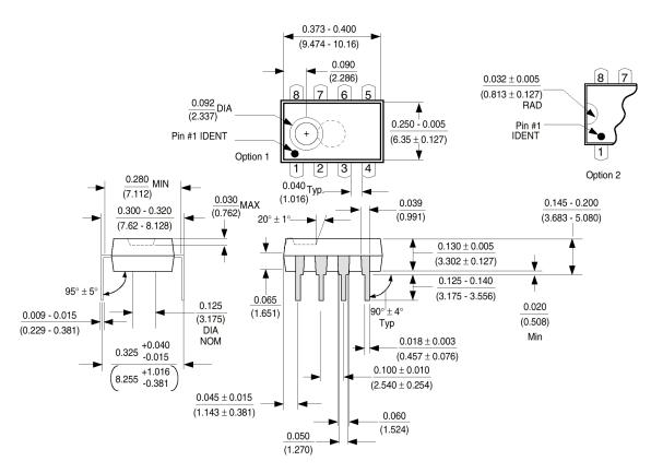
Figure 31. Molded Dual-in-line Package (N) Package Number N08E
