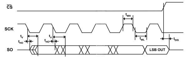
Figure 5. SPI Mode 0 (0,0) Output Timing
