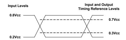
Figure 6. AC Measurements I/O Waveform
