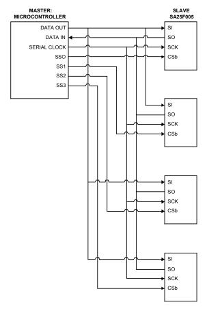
Figure 9. SPI Serial Interface
