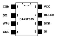
Figure 2. SOIC 8 (150 mil)/PDIP/MLF Package (Top View)
