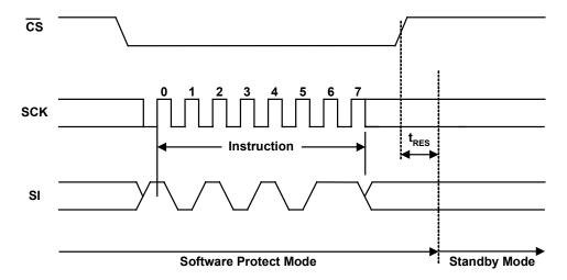
Figure 25. Release from Software Protect (RES) Instruction Sequence
