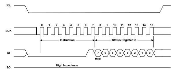
Figure 13. Write Status Register (WRSR) Instruction Sequence
