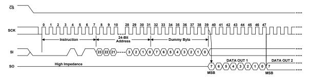
Figure 15. Fast Read (FAST READ) Instruction Sequence
