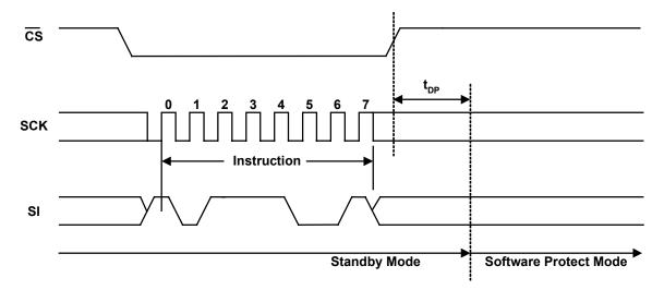
Figure 24. Software Protection Instruction Sequence
