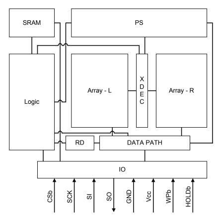
Figure 1. SA25F005 Block Diagram
