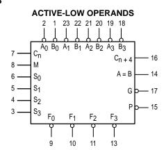
V<sub>CC</sub> = PIN 24 GND = PIN 12
