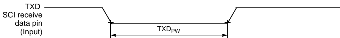
Figure 10-17 TXD Pulse Width
