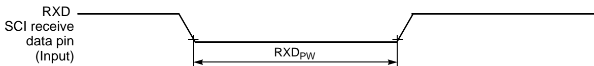
Figure 10-16 RXD Pulse Width
