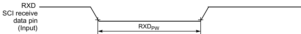
Figure 10-15 RXD Pulse Width
