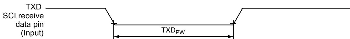
Figure 10-16 TXD Pulse Width
