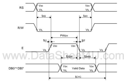
Fig.1 Write Operation Timing
