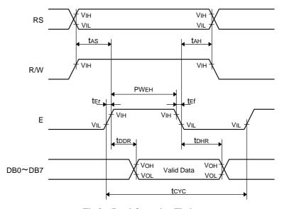
Fig.2 Read Operation Timing
