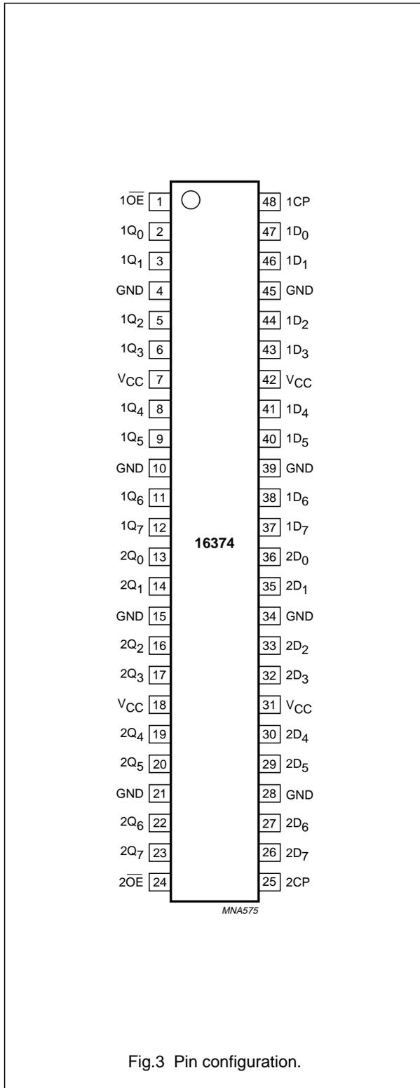
Fig.3 Pin configuration.
