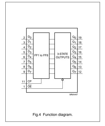
Octal D-type flip-flop; positive edge-trigger; 3-state
