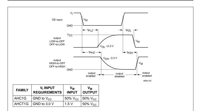
Fig.6 The 3-state enable and disable times.
