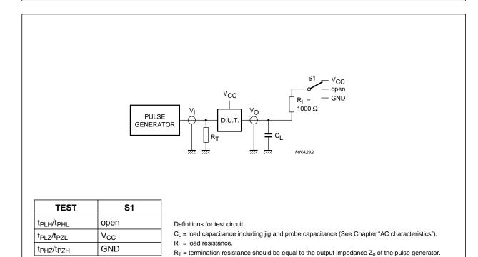
Fig.7 Load circuitry for switching times.
