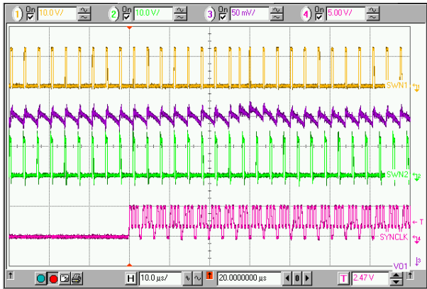
Top to Bottom: SWN_Slave, Vo_Slave, SWN_Master, Sync_clk
