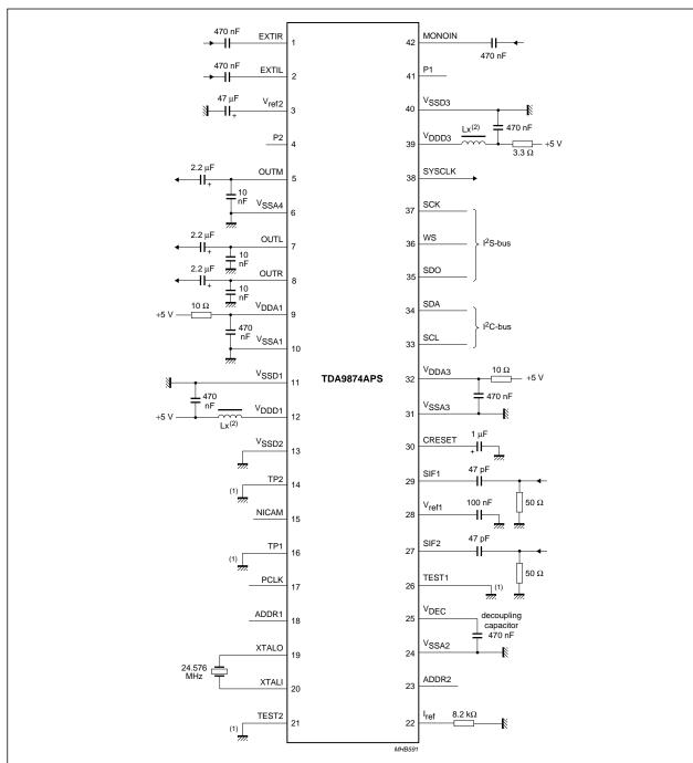
All analog and digital supply ground pins are connected internally and should be connected via a massive external ground plate.
