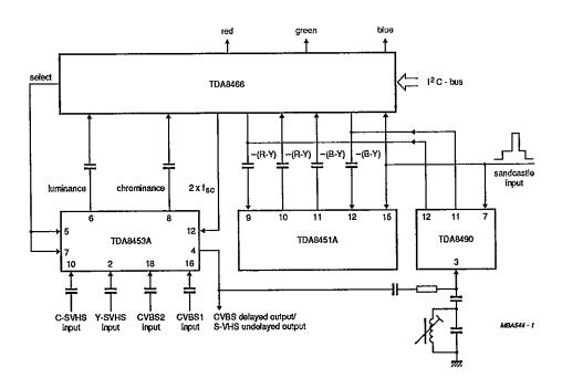
Fig.3 PAL-NTSC-SECAM decoder configuration.
