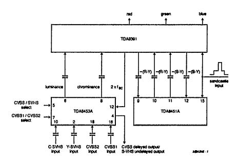
Fig.2 PAL decoder configuration.
