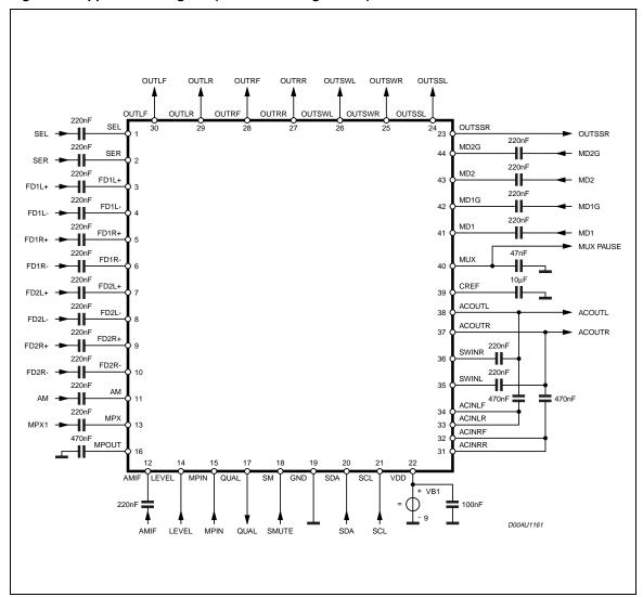
Figure 33. Application Diagram (Dual MPX mode)
