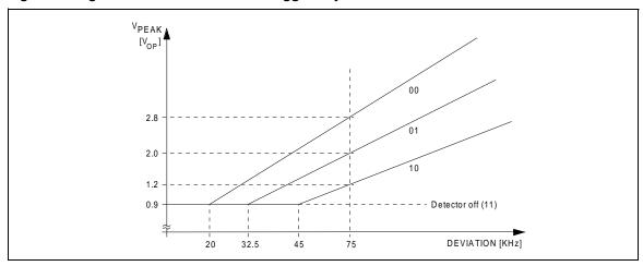
Figure 22. Fieldstrength Controlled Trigger Adjustment
