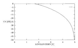
The gain can be programmed through 4 bits in the "Stereodecoder-Adjustment"-byte. All necessary internal reference voltages like REF5V are derived from a bandgap circuit. Therefore they have a temperature coefficient near zero.
