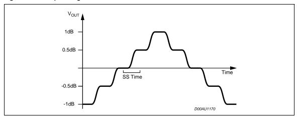
Note: For steps more than 0.5dB (Volume) /1dB (speaker) the SoftStep mode should be deactivated because it could generate a hard 1dB step during the blend-time.
