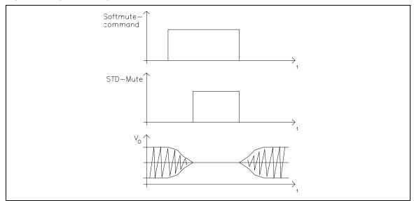
Figure 24. Signals during stereodecoder's SoftMute
