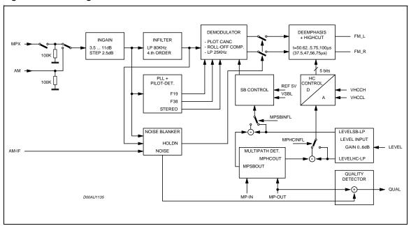
The stereodecoder-part of the A679 (see Fig. 23) contains all functions necessary to demodulate the MPX-signal like pilottone-dependent MONO/STEREO-switching as well as "stereoblend" and "highcut". Adaptations like programmable input gain, roll-off compensation, selectable deemphasis time constant and a programmable fieldstrength input allow to use different IF-devices.
