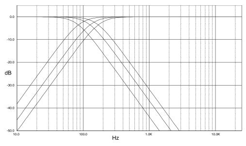
Both filters, the lowpass- as well as the highpass-filter, have butterworth characteristic so that their cut-off frequencies are not equal but shifted by the factor 1.125 to get a flat frequency response.
