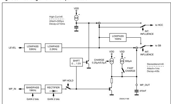
Figure 30. Blockdiagram of the Multipath-Detector
