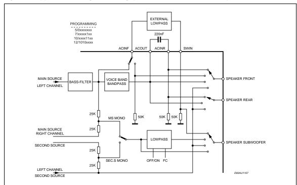
Figure 17. Application2 using internal Highpass- and external stereo Low-pass-Filter
