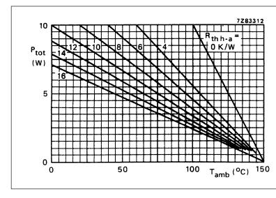
Fig.2 Total power dissipation.  $R_{th\ h-a} \text{ includes } R_{th\ mb-h}$  which is expected when heat-sink compound is used.  $R_{th\ j-mb} \leq 5 \text{ K/W}.$
