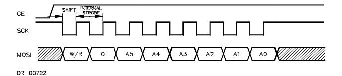
**Read/Write Data:** The Read/Write Data follows the Address/Control byte. SCK may be either polarity.
