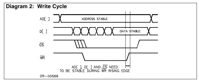
The Write cycle timing diagram is given below:
