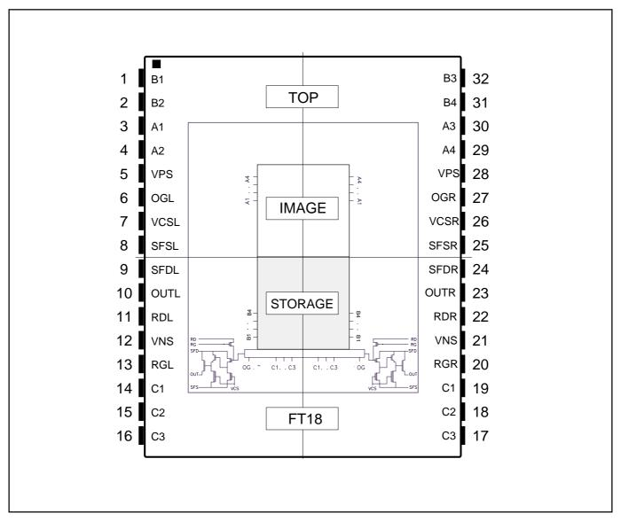
Figure 7 - FT18 pin configuration (top view)
