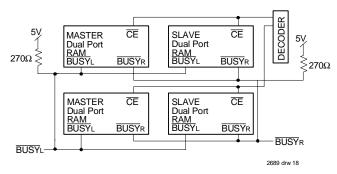
Figure 3. Busy and chip enable routing for both width and depth expansion with IDT7130 (Master) and IDT7140 (Slave)RAMs.
