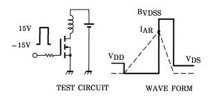
$$\begin{array}{ll} \text{Peak I}_{AR}\!=\!2\text{A, R}_{G}\!=\!25\Omega & \text{E}_{AS}\!=\!\frac{1}{2}\!\cdot\!\text{L}\!\cdot\!\text{I}^{2}\!\cdot\!(\frac{\text{BVDSS}}{\text{BVDSS-V}_{DD}}) \end{array}$$
