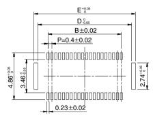
Recommended solder paste thickness: 120  $\mu m$
