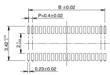
Recommended solder paste thickness: 120  $\mu$ m
