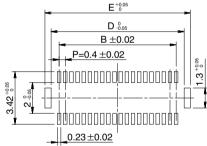
Recommended solder paste thickness: 120  $\mu m$
