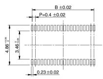
Recommended solder paste thickness: 120  $\mu m$
