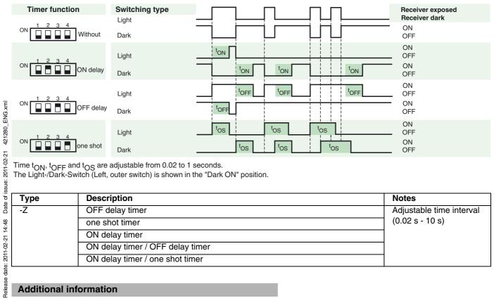
Time  $t_{ON}$ ,  $t_{OFF}$  and  $t_{OS}$  are adjustable from 0.02 to 1 seconds.
