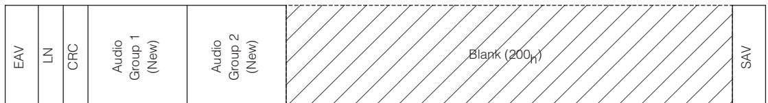
Video Signal after GS1503B Insertion of Audio Groups 1 & 2 (CASCADE = 0)
