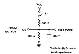
This is the A.C. Test Load which Harris Semiconductor uses in its automatic test equipment, and it is recommended that users of Harris bipolar devices use the same or an equivalent load in performing A.C. testing.
