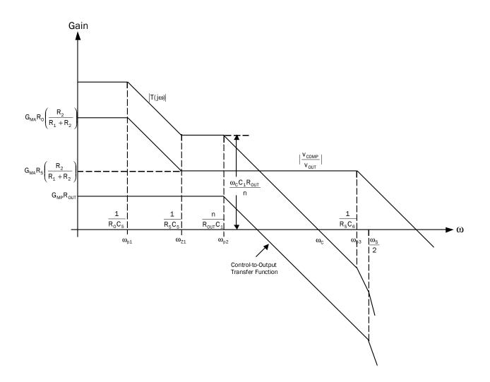
Figure 12. Bode Plots of Control-to-Ouput, Output-to-Control and the Overall Loop Gain. Control-to-output transfer function is shown with two poles near half the switching frequency  $\omega_s$ .
