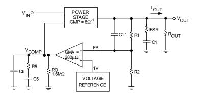
Figure 11. Simplified Control Loop Equivalent Circuit
