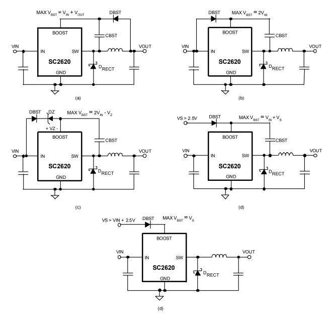
Figure 7. Methods of Bootstrapping the SC2620.
