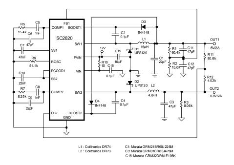
Figure 17(a). 500kHz 12V to 5V and 0.8V step-down converter. Notice that  $V_{0UT2}$  is lower than the nominal FB voltage.  $R_{11}$  and  $R_{12}$  constitute the feedback voltage divider for Channel 2.
