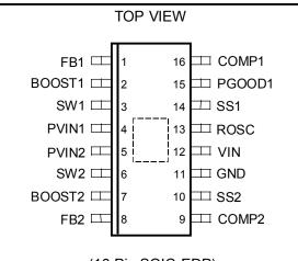
(16 Pin SOIC-EDP) Underside metal must be soldered to ground.
