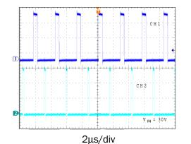
CH1 : SW1 Voltage, 10V/div CH2 : SW2 Voltage, 10V/div
