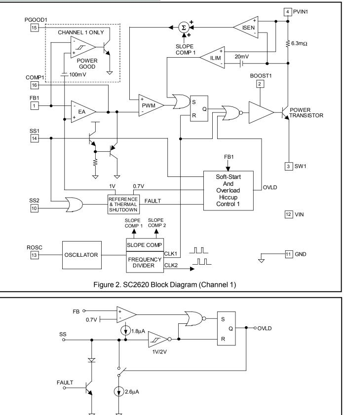
Figure 3. Details of the Soft-Start and Overload Hiccup Control Circuit
