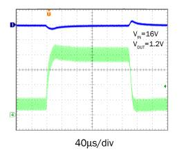
Upper Trace : OUT2 Voltage, AC Coupled, 0.5V/div Lower Trace :  $L_2$  Inductor Current, 0.5A/div
