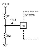
Figure 4. V<sub>out</sub> is set with a Resistive Divider
