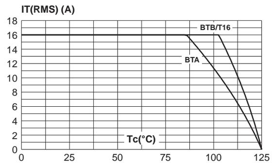
**Fig. 2-2:** D<sup>2</sup>PAK RMS on-state current versus ambient temperature (printed circuit board FR4, copper thickness: 35 μm), full cycle.
