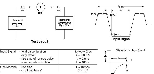
\*C = oscilloscope input capacitance + parasitic capacitance
