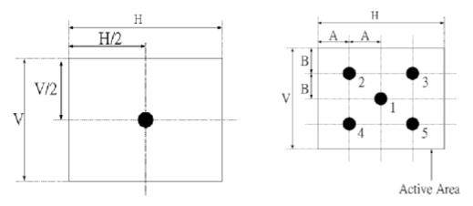
Fig.4-2 Optical measurement point
