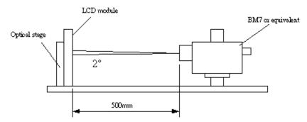
Fig.4-1 Optical measurement equipment and method
