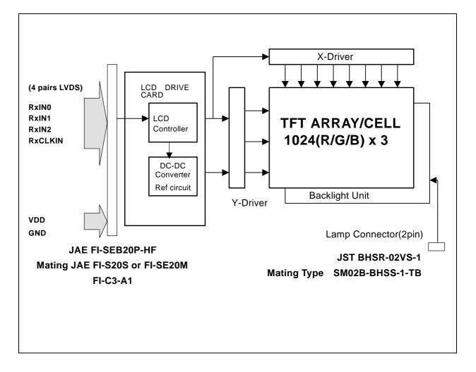
The following diagram shows the functional block of the 14.1 inches Color TFT/LCD
